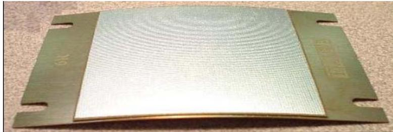
Fig 2. TH-6R Piezo Electric Sensor [5].
